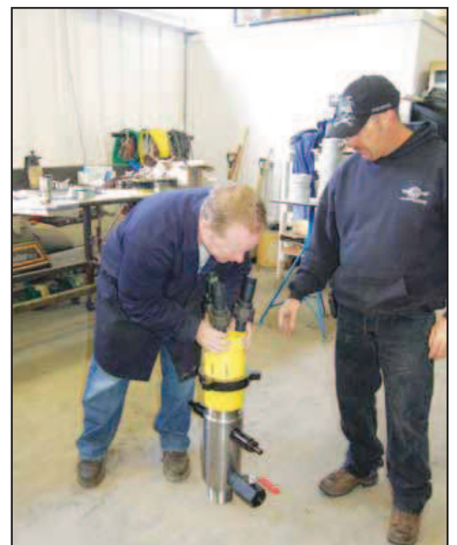
Collin Morris fits the terminator cap to a wellhead made for the CJS FLATpak coil tubing while Joe Reck looks on.
