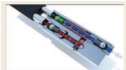
Fig. 9. Two check valves are the only moving parts in the VLift closed-loop, single-point gas lift system.
