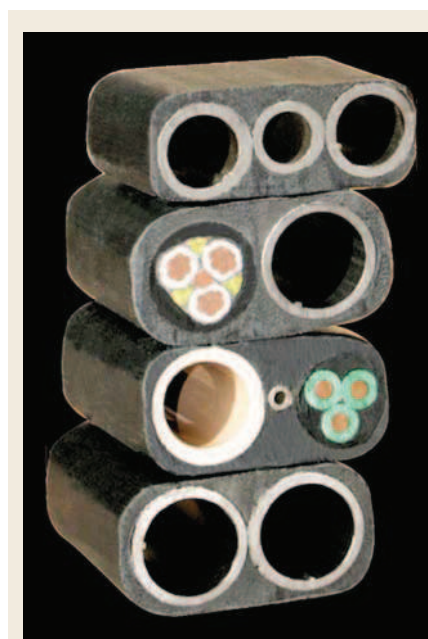
Fig. 1. CJS Coiled Tubing Supply's conveyance system for deliquification systems encapsulates multiple coiled tubing strings or electrical conduits of different sizes in a high-strength thermoplastic jacket.
