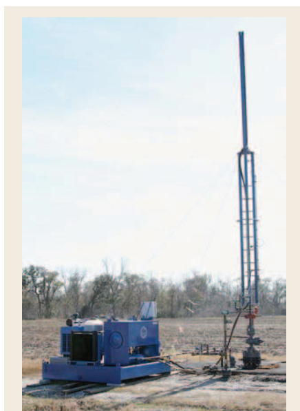
Fig. 6. Petro Hydraulic Lift Systems’ innovative pumping unit replaces traditional horsehead pumps in rod pumping applications, with reduced rod and tubing wear and increased production efficiency.
