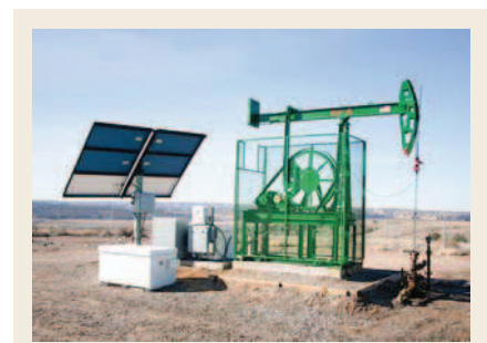
Fig. 8. The Low-Volume Pumping System incorporating the Eco² pumping unit and continuous fiberglass rod can use solar power to dewater low-volume wells with very low horsepower requirements.
